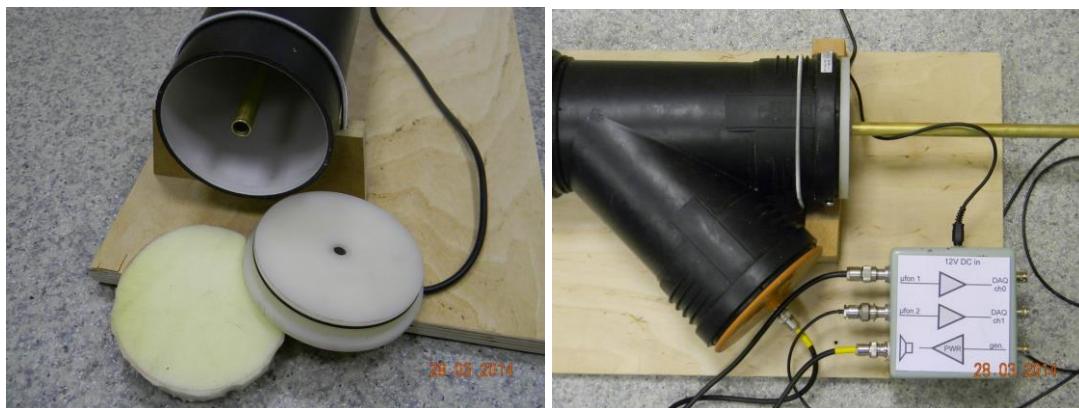
Fig. 13. (left): The plastic end-wall or stopper with the microphone in the middle, sealed by a black O-ring; A sponge sample; The open end of the tube with the tip of the microphone-slider;
