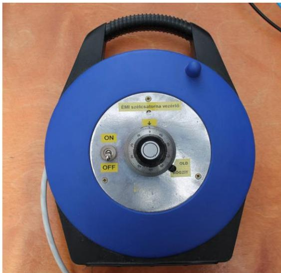
**Fig. 2.** The wind tunnel controller with a 10-turn potentiometer.
