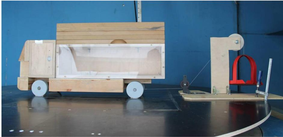
**Fig. 5.** The guide pulleys and the calibration basket. (Weight: 0.7527kg).
