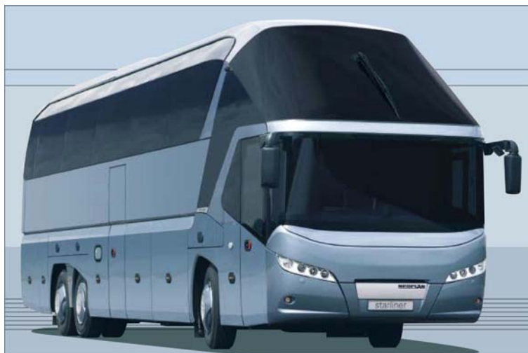
Figure 22 – German-designed intercity bus with C_D \approx 0.35 .
