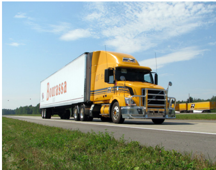
Figure 10 – Heavy duty bumper mounted to a tractor
