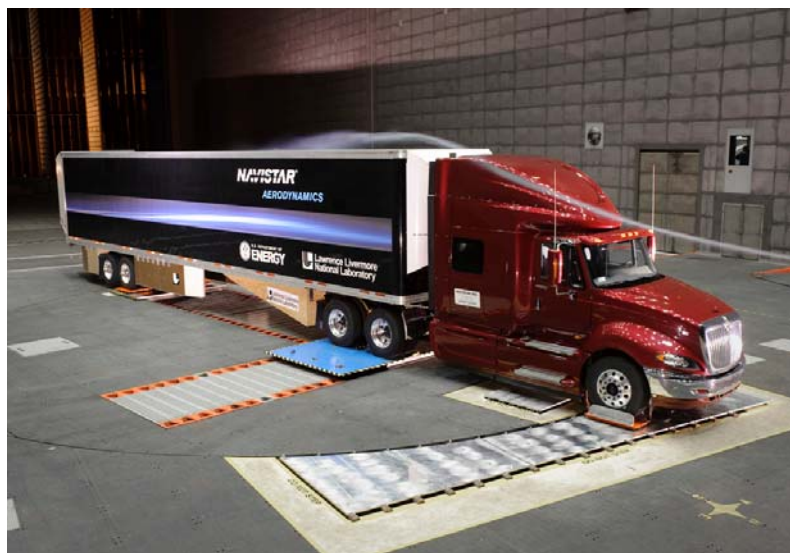
Figure 25 – Full-scale tractor-trailer testing in the NFAC 24 m x 36 m Wind Tunnel
