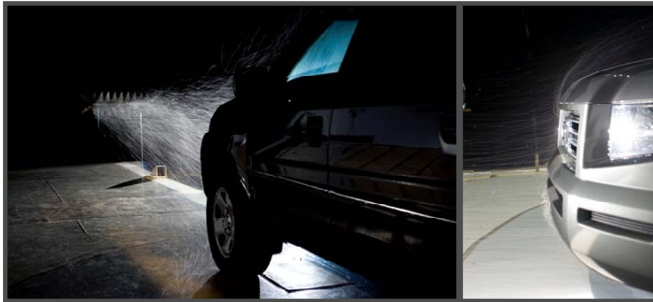
Figure 31 – Snow-storm simulation in 9 m x 9 m Wind Tunnel
