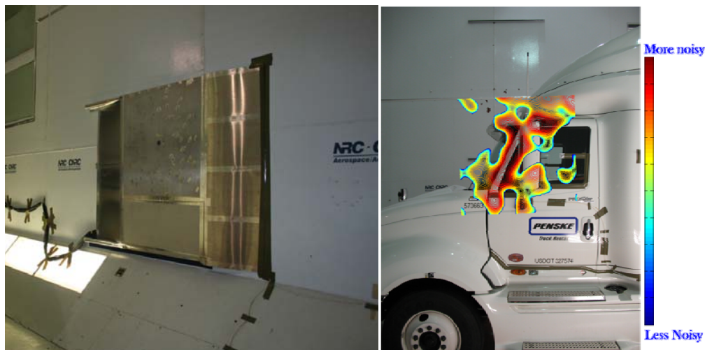
Figure 30 – NRC aero-acoustic array mounted to side-wall of 9 m x 9 m Wind Tunnel (left) and subset of preliminary acoustic measurements for a tractor (right).
