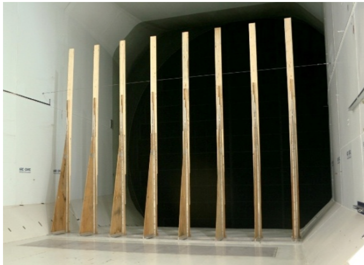
Figure 29 – Partial-height turbulence grid in NRC 9 m x 9 m Wind Tunnel
