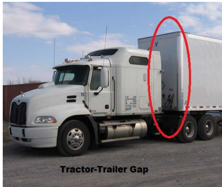
Figure 13 – Typical tractor-trailer gap
