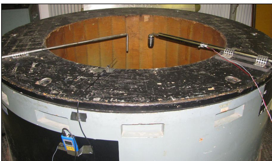
Fig.2.2. Reference Pitot-static tube (left) and KS-412-w1_50 type sampling probe (right) in the test section
