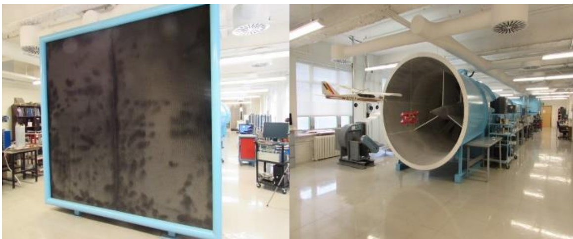
Figure 14 top) Schematic diagram of wind tunnel bottom left) Inlet of the wind tunnel, and bottom right) acoustic silencer of the wind tunnel
