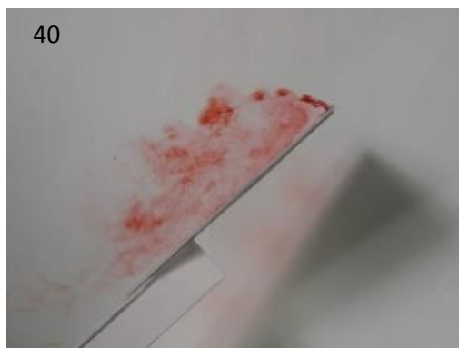
Figure 26 Dye flow visualization (middle injection) of RDW at \alpha = 10^\circ - 40^\circ
