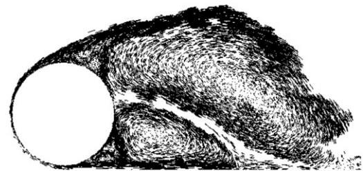
Fig. 16. Near wake behaviour using moving ground at an instant represented by point C for h/d=0.05 .
