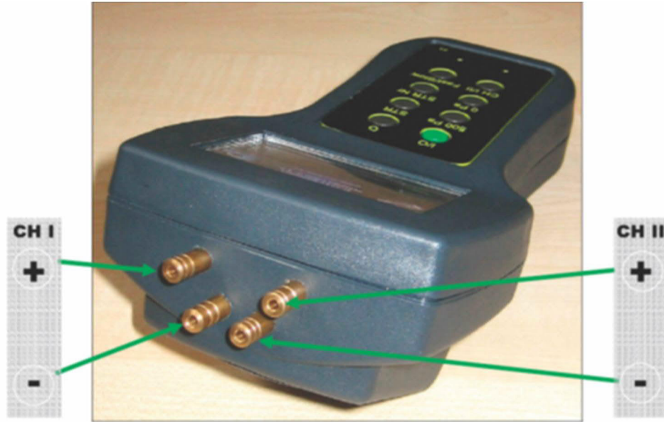
Fig.9.: Digital manometer EMB-001 type
