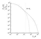
Recall: the cutting wavenumber ( $\kappa_c$ ), below which modelling is needed
