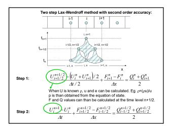
This is an explicit time marching scheme. Only conditionally stable. According to the linear stability theory:
