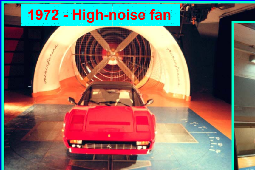
1972 - No Acoustic Treatment on the plenum walls
