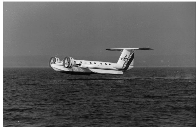
Figure 2. A WIG aircraft flying over water (courtesy of WIG Vehicle Development Center of Chinese Academy of Science & Technology Development).
