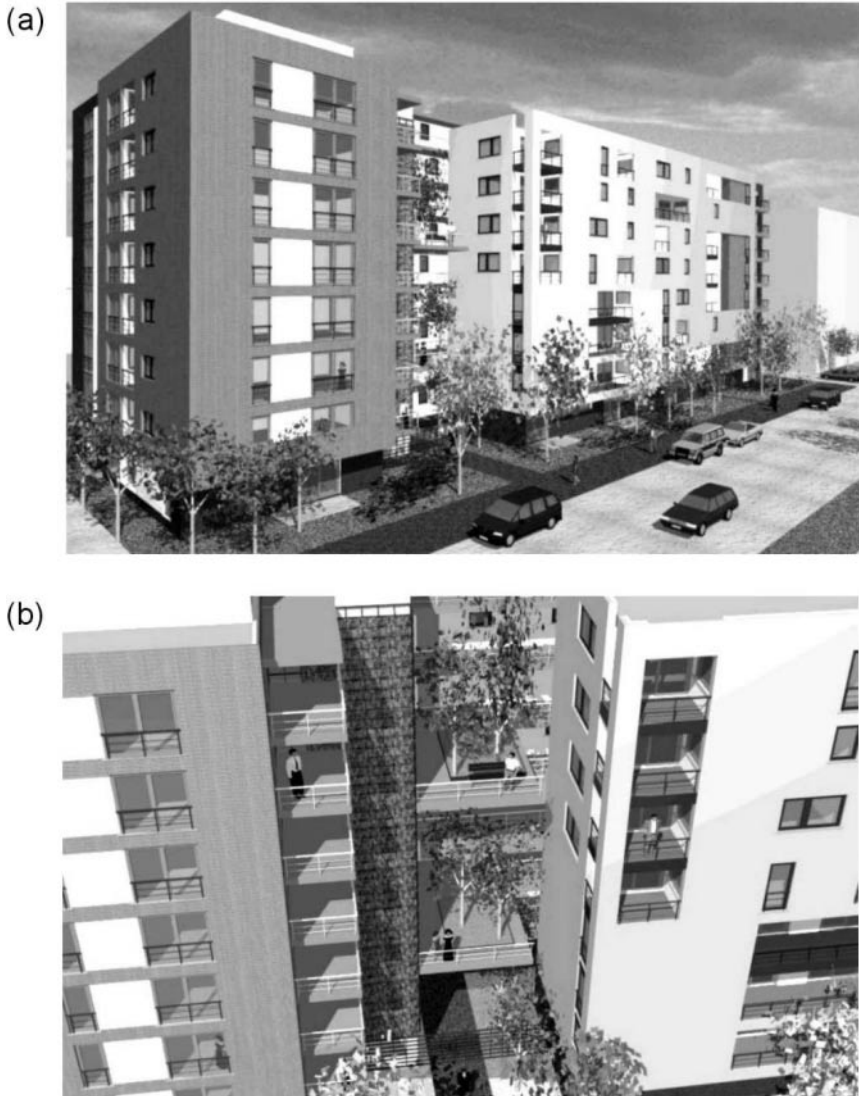
Figure 23. Perspective view of the proposed design for residence “Joan Miro”: (a) The building has dimensions L \times B \times H = 61 \times 22 \times 26 \text{ m}^3 and consists of nine floors; (b) At each floor, the apartments are accessible through the use of outdoor pedestrian platforms. The platforms connect the individual apartments with the staircases and elevators (reproduced with permission, © Herelixka and Claesen, 2003).
