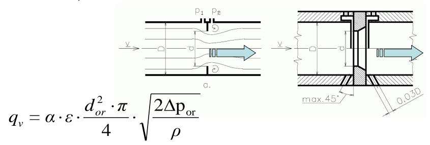
$\beta = d/D$  Cross-section ratio
