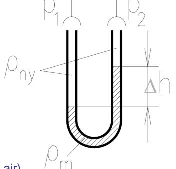
Density of the measured fluid:  $\rho_{nv}$  (For example air)
