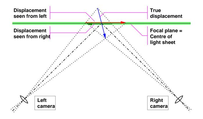
True 3D displacement ( $\Delta X$ ,  $\Delta Y$ ,  $\Delta Z$ ) is estimated from a pair of 2D displacements ( $\Delta x$ ,  $\Delta y$ ) as seen from left and right camera respectively
