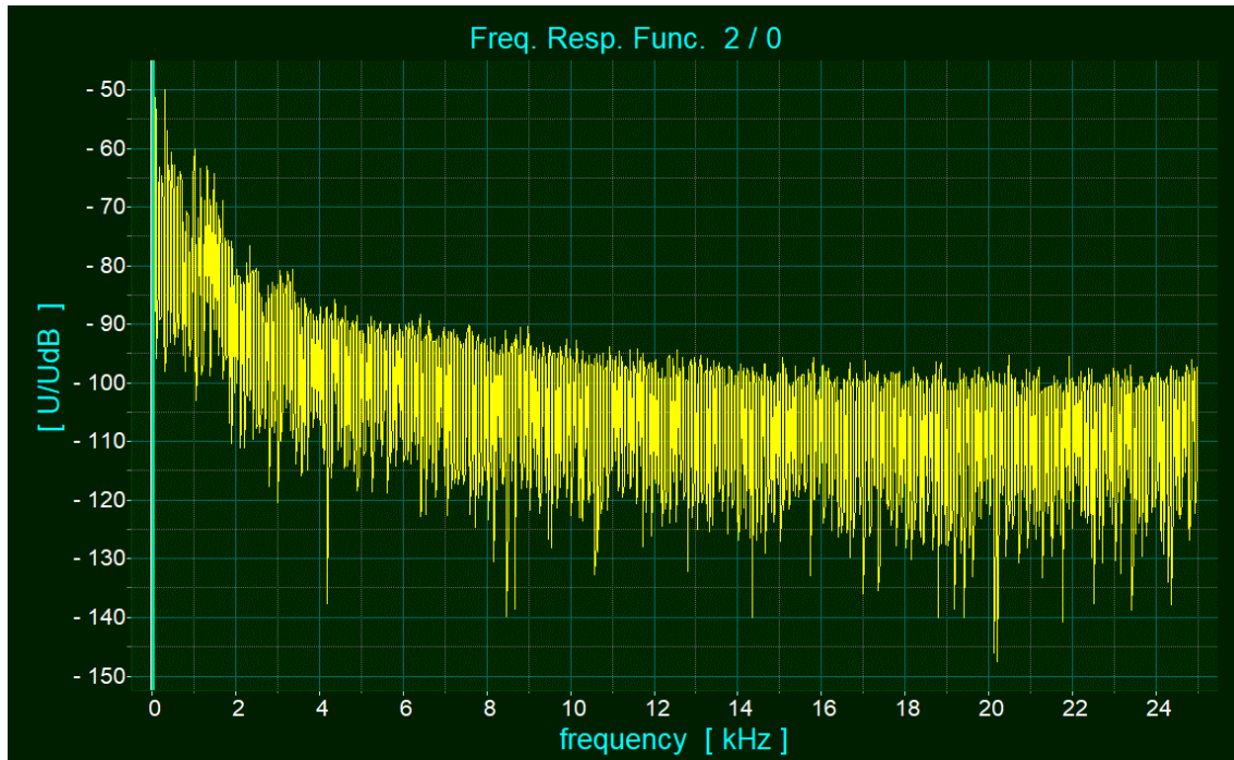
Figure 8: Sound level measurement – perfect box condition
