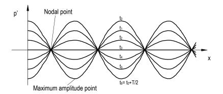
The graph of the sound pressure in a standing wave function versus distance in different time
