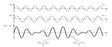
The sound pressure distribution of the components and resultant waves of a beat in time, at x= 0m position
