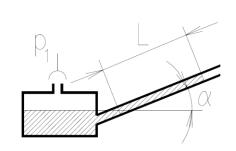
$$\frac{\delta L}{L} = \frac{\delta L}{\frac{\Delta h}{\sin \alpha}} = \frac{1mm}{\frac{10mm}{\sin 30^{\circ}}} = 0.05 = 5\%$$
