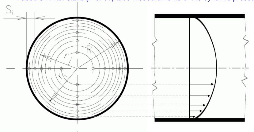
This is a standardized procedure, and the measurement point are given in the standard (MSZ 21853/2):
