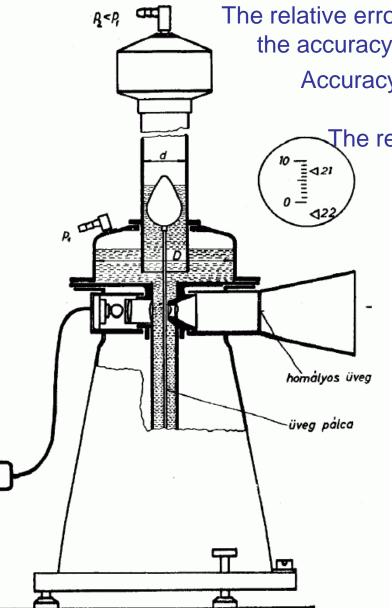
The relative error is reduced by optical means, improving the accuracy.
