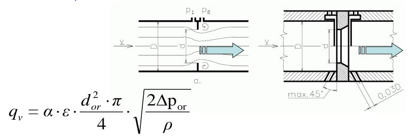
$\beta = d/D$  Cross-section ratio
