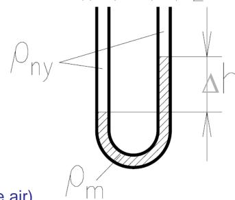
Density of the measured fluid:  $\rho_{nv}$  (For example air)
