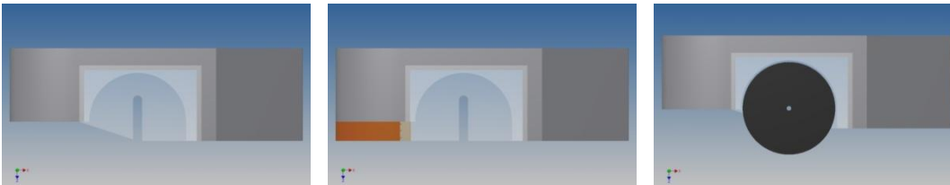
Effect of adding wheel to basic faired body
