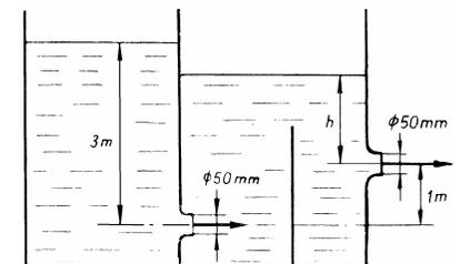
4/20 Determine the quotient of the flow rates with and without horizontal plate!
