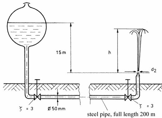
5/17 Water of  $q_v = 18 \text{ m}^3/\text{h}$  flow rate has to be transported by the equipment shown in the figure.
