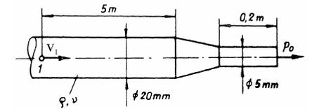
5/3 Friction loss of the transitional section is negligible.
