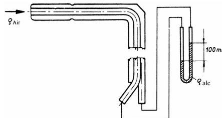
3/16 The inner diameter of an orifice flowmeter is  $d = 200 \text{ mm}$ . Flow coefficient  $\alpha = 0.7$
