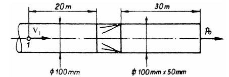
5/4 How do the Reynolds number and the pressure loss of a straight, smooth pipe depend on diameter in case of laminar and turbulent flow, if the flow rate is constant?
