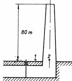
1/5 The figure shows a vertical section of a gas pipe. At the lower tap there is an overpressure of 500 Pa. How big is the overpressure at the upper tap?
