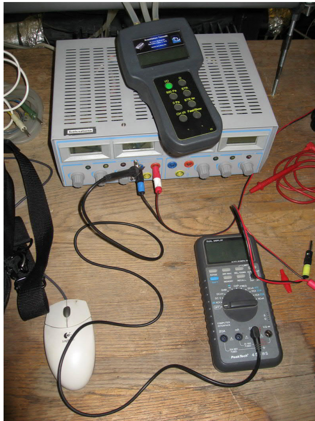
Figure 3, Manometer, Voltage Source and Digital Multimeter
