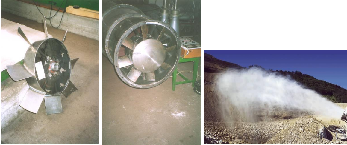
Fig. 2.1. The prototype of the axial fan of high throwing distance (used in fog cannons) with sheet metal blades and bluff hub nose. Developed at the Department of Fluid Mechanics, Budapest University of Technology and Economics.
