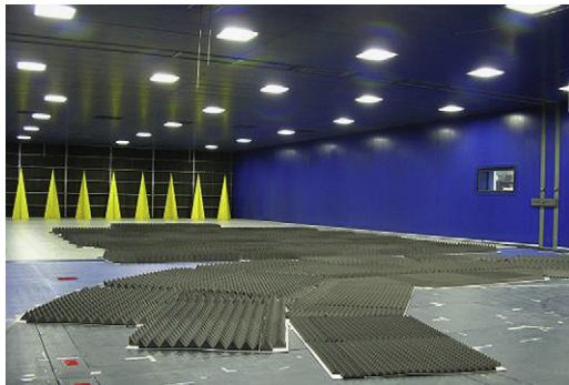
Fig. 6. Wind tunnel experimental set-up: boundary layer simulation.
