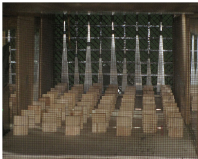
Figure 5.2: The adjustment of obstacles and spikes, and the measuring arrangement
