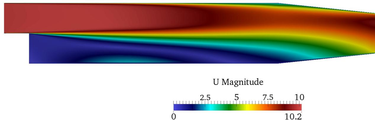
LES turbulence: UMean field (time-averaged velocity)
