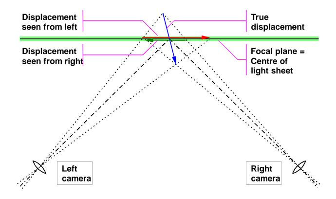
True 3D displacement ( $\Delta$  X,  $\Delta$  Y,  $\Delta$  Z) is estimated from a pair of 2D displacements ( $\Delta$  x,  $\Delta$  y) as seen from left and right camera respectively
