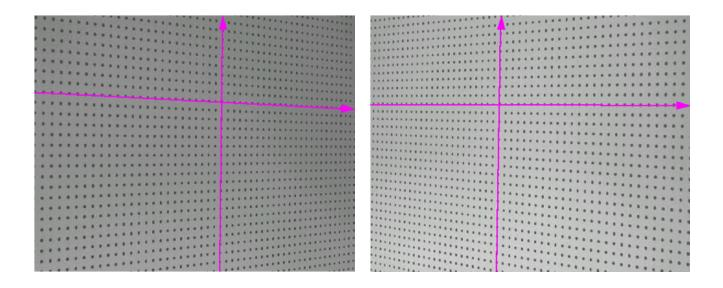
Images of a calibration target are recorded.
