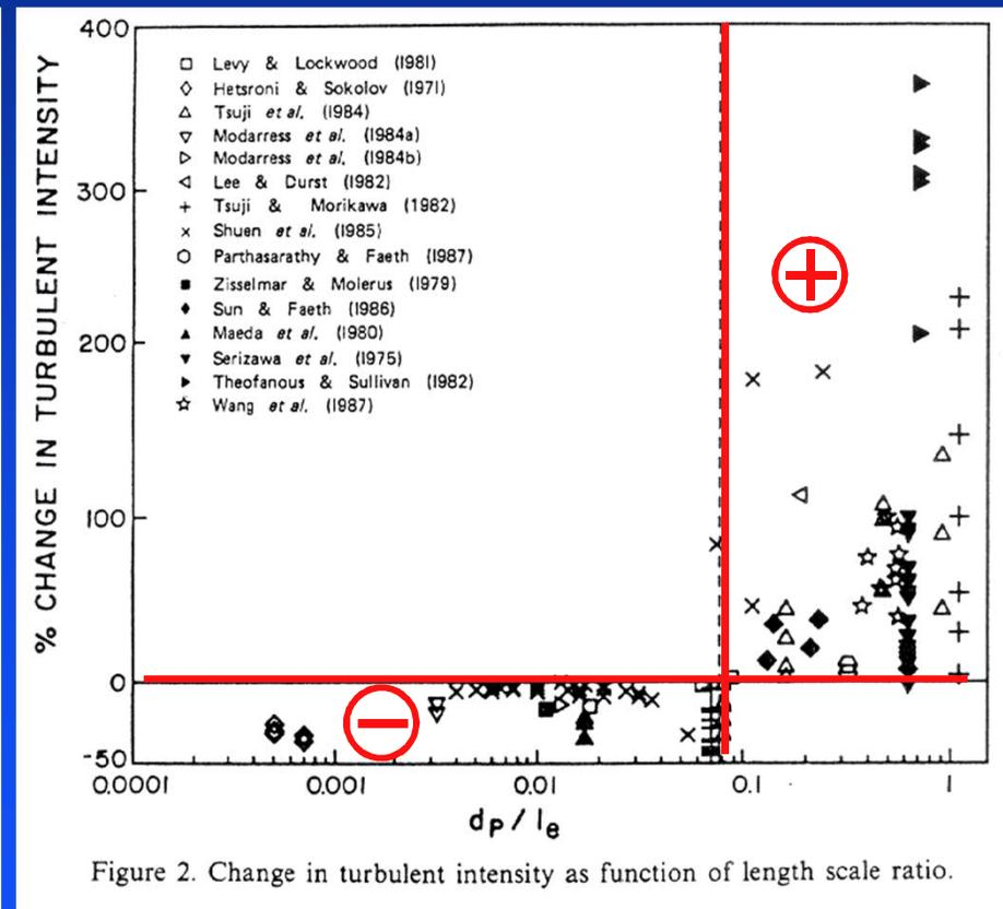
Figure 2. Change in turbulent intensity as function of length scale ratio.
