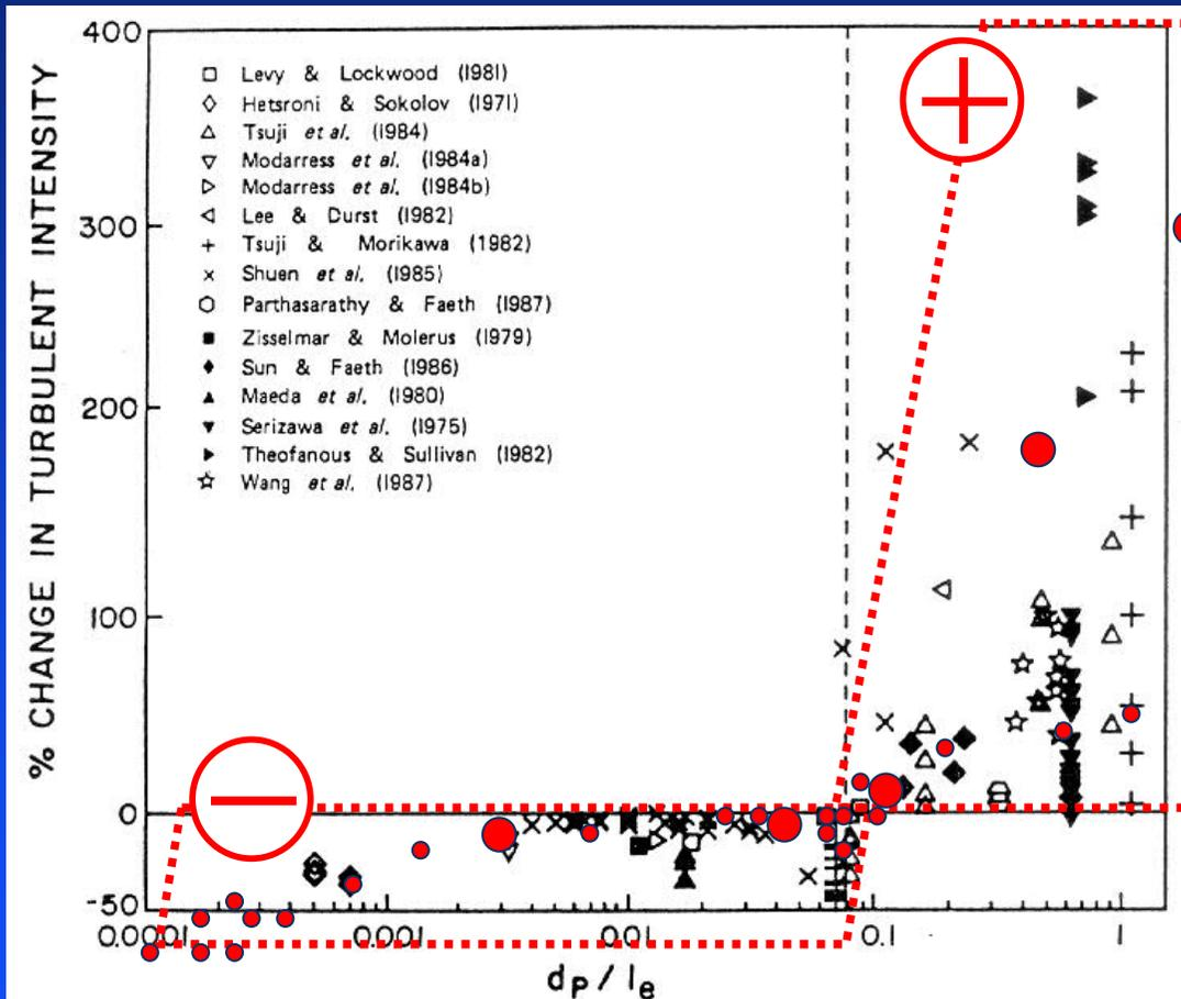
● Effect of characteristic length scale ratio on modulating turbulent intensity:
