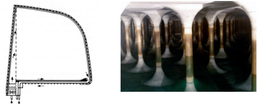
2 piano shaped reservoirs 40.000 m 3 each.
