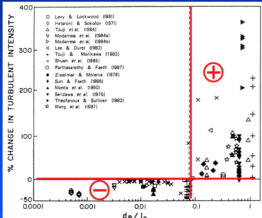
Figure 2. Change in turbulent intensity as function of length scale ratio.
